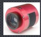
1) Higher Resolution since all pixel are recording image luminosity no Bayer Filter
